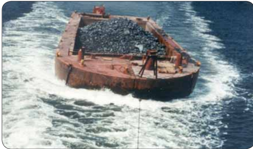
A hopper scow loaded with dredge rock material on its way to the reef.
